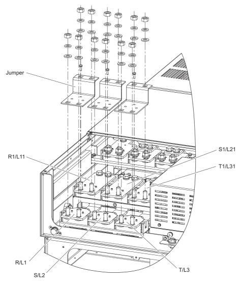
Figure 3.2 Removing the Jumper
