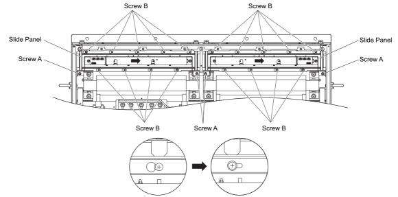
Figure 7.42 Removing the Fan Unit: 4A0930 and 4A1200
