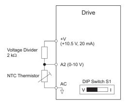
Figure 5.64 Motor Protection Circuit using NTC Input
