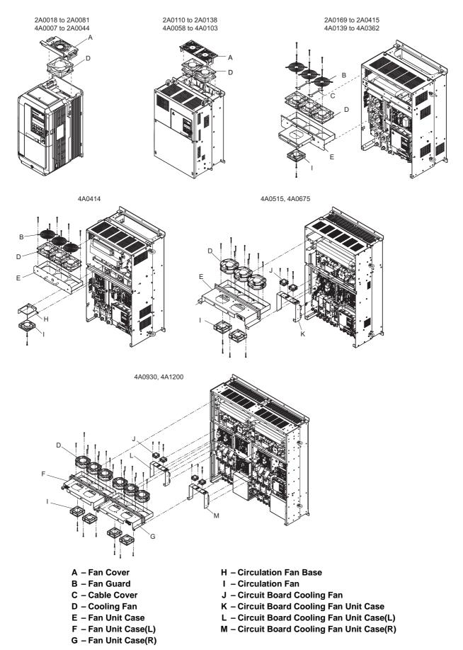
Figure 7.1 Cooling Fan Component Names
