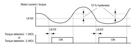
Figure 5.79 Undertorque Detection Operation
