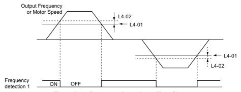
Figure 5.44 Frequency Detection 1 Time Chart
