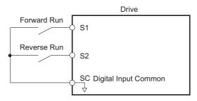
Figure 5.38 Example Wiring Diagram for 2-Wire Sequence
