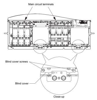
Figure 7.51 Air Filter Replacement: Removing the Blind Cover
