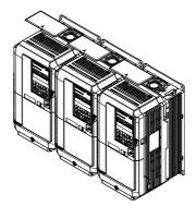
Figure 2.4 IP20/NEMA 1, UL Type 1 Side-by-Side Mounting in Enclosure
