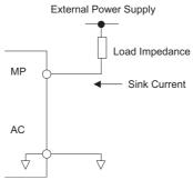
Figure 3.32 Pulse Output Connection Using External Voltage Supply
