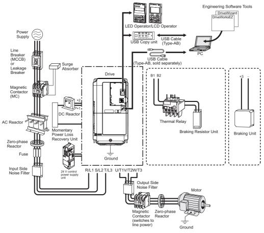
Figure 8.1 Connecting Peripheral Devices
