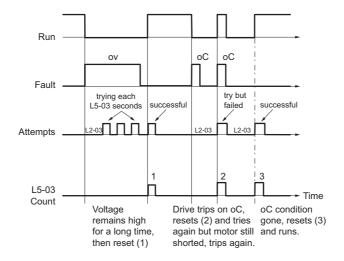
Figure 5.77 Automatic Restart Timing Diagram
