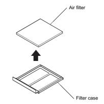
Figure 7.54 Air Filter Replacement: Taking Out the Filter
