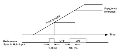
Figure 5.37 Analog Frequency Reference Sample/Hold
