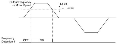
Figure 5.49 Frequency Detection 4 Example with Positive L3-04 Value
