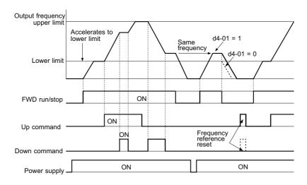
Figure 5.34 Up/Down Command Operation
