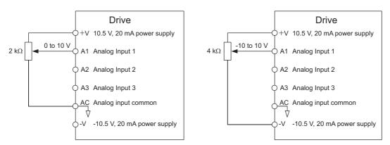
Figure 5.1 Setting the Frequency Reference as a Voltage Signal at Terminal A1
