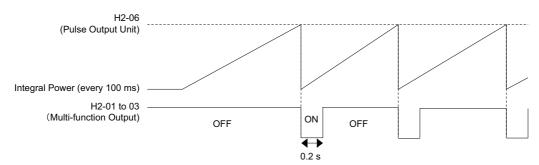
Figure 5.52 Watt Hour Output Example
