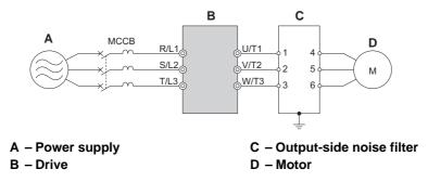
Figure 8.15 Output-Side Noise Filter
