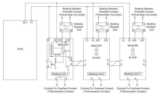
Figure 8.10 Connecting Braking Units in Parallel
