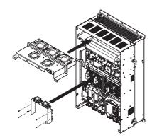
Figure 7.40 Installing the Cooling Fan Units: 4A0515 and 4A0675
