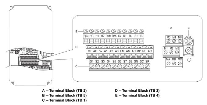
Figure 3.24 Control Circuit Terminal Arrangement
