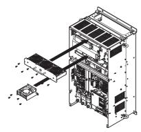
Figure 7.30 Installing the Cooling Fan Unit: 4A0414
