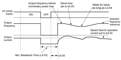
Figure 5.10 Current Detection Speed Search after Power Loss
