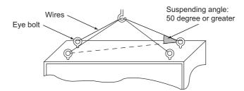
Figure 2.6 State of Suspension with Wires
