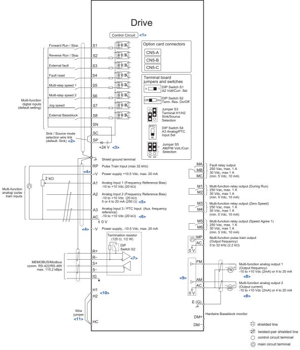
Figure 3.22 Control Circuit Connection Diagram
