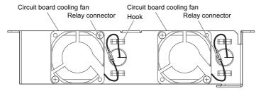
Figure 7.39 Cooling Fan Wiring: 4A0515 and 4A0675
