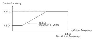
Figure 5.22 Carrier Frequency Changes Relative to Output Frequency
