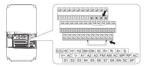
Figure C.9 Terminal Connections for Communication Self-Diagnostics
