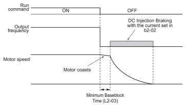
Figure 5.4 DC Injection Braking to Stop
