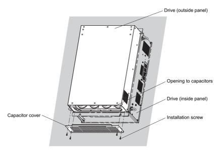
Figure D.8 Capacitor Cover (2A0110 to 2A0415, 4A0068 to 4A0675)
