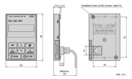
Figure 2.8 Digital Operator Dimensions
