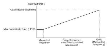
Figure 5.7 Run Wait Time Depending on Output Frequency
