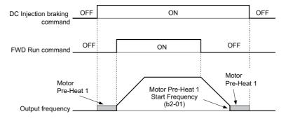
Figure 5.39 DC Injection Braking Input Timing Diagram
