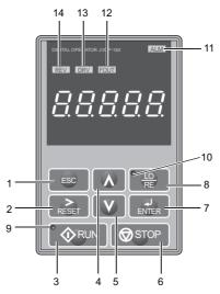
Figure 4.1 Keys and Displays on the Digital Operator
