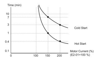
Figure D.7 Motor Overload Protection Time
