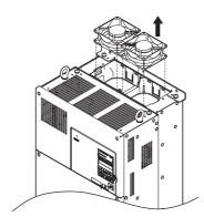
Figure 7.14 Removing the Cooling Fan: 4A0088 and 4A0103
