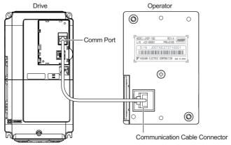
Figure 2.7 Communication Cable Connection
