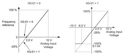
Figure 5.54 Frequency Reference Setting by Analog Input with Negative Bias
