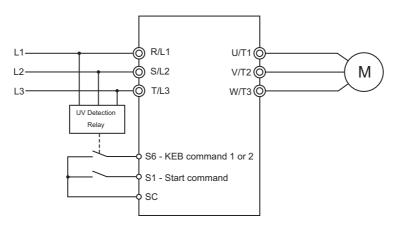
Figure 5.71 KEB Function Wiring Example
