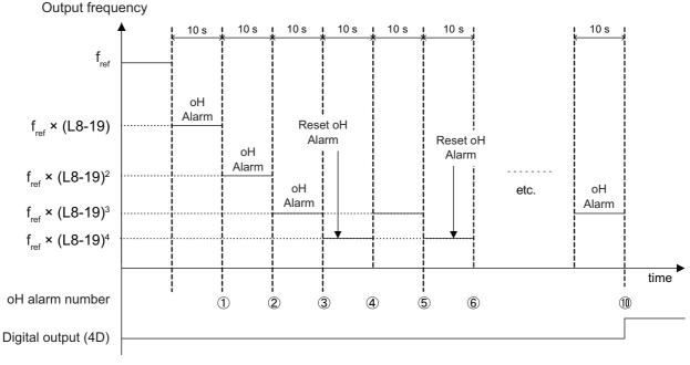
Figure 5.81 Output Frequency Reduction During Overheat Alarm
