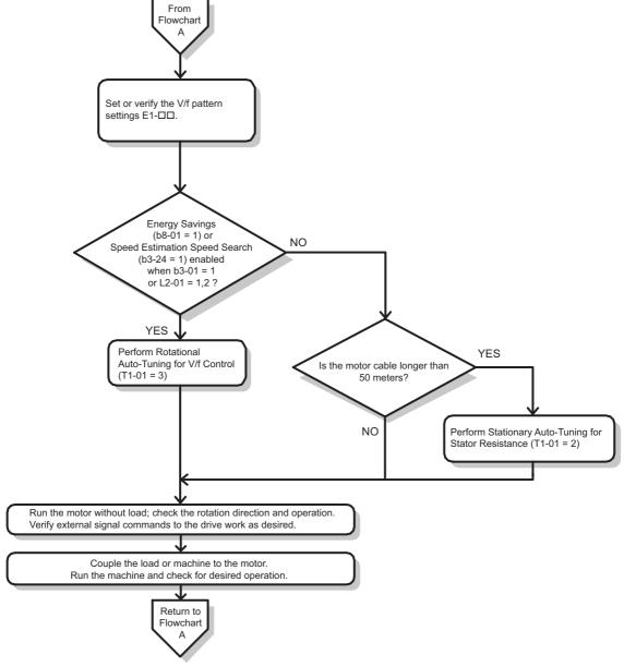
Figure 4.8 Simple Motor Setup with Energy Savings or Speed Search
