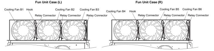
Figure 7.45 Cooling Fan Wiring: Models 4A0930 and 4A1200
