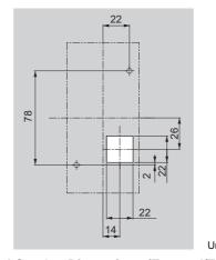
Figure 2.10 Panel Cut-Out Dimensions (External/Face-Mount Installation)
