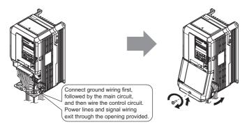
Figure 3.7 Reattaching the Terminal Cover on an IP20/NEMA 1, UL Type 1 Enclosure Drive
