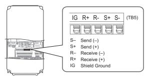
Figure C.2 Serial Communications Cable Connection Terminals (TB5)
