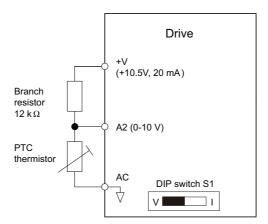
Figure 5.62 Connection of a Motor PTC
