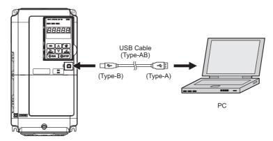
Figure 3.34 Connecting to a PC (USB)
