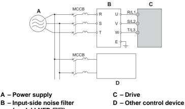
B - Input-side noise filter (model LNFD-□□)
