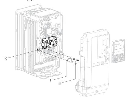
Figure 8.6 Connect the Ground Wire
