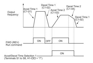
Figure 5.19 Timing Diagram of Accel/Decel Time Change
