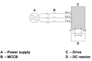
Figure 8.13 Connecting a DC Reactor
