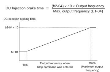
Figure 5.5 DC Injection Braking Time Depending on Output Frequency
