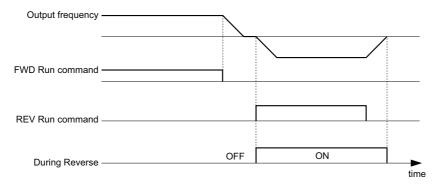
Figure 5.50 Reverse Direction Output Example Time Chart
