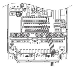
Figure 3.27 Terminal Board Wiring
