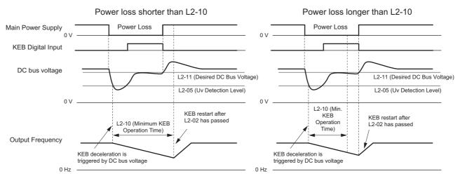
Figure 5.70 KEB Operation Using L2-10 and KEB Input
