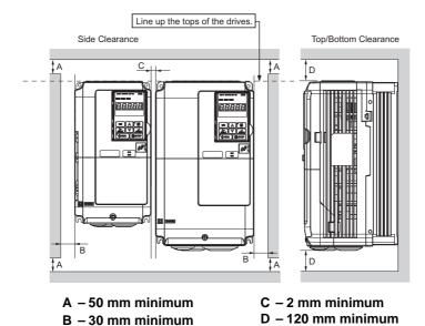
Figure 2.3 Space Between Drives (Side-by-Side Mounting)
