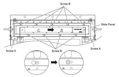
Figure 7.32 Removing the Fan Unit: 4A0515 and 4A0675
