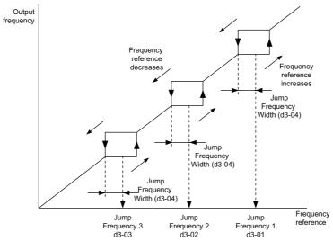
Figure 5.26 Jump Frequency Operation
