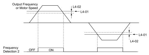
Figure 5.45 Frequency Detection 2 Time Chart
