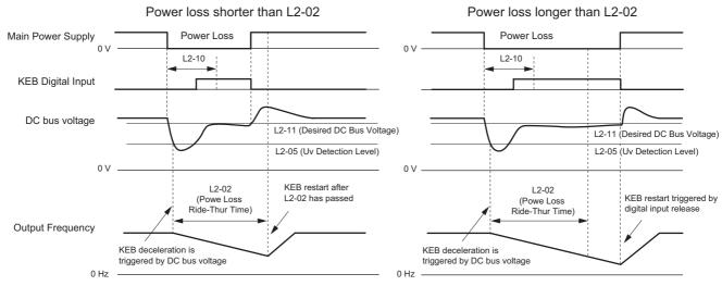
Figure 5.68 KEB Operation Using L2-02 and KEB Input
