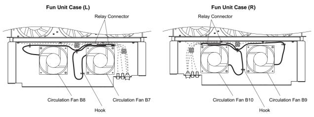
Figure 7.47 Cooling Fan Wiring: Models 4A0930 and 4A1200
