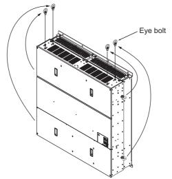
Figure 2.5 Attaching Eye Bolts on Top Panel
