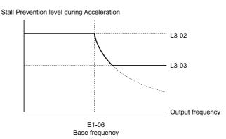
Figure 5.74 Stall Prevention Level and Limit During Acceleration
