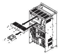
Figure 7.27 Removing the Fan Unit: 4A0414
