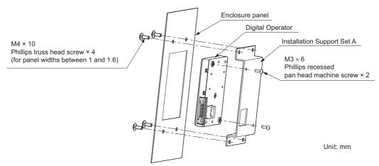
Figure 2.11 Internal/Flush Mount Installation
