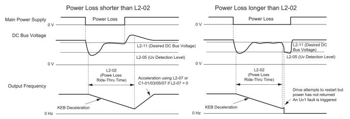
Figure 5.67 KEB Operation Using L2-02, Without KEB Input
