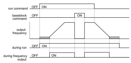
Figure 5.51 During Frequency Output Time Chart
