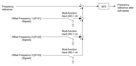
Figure 5.28 Offset Frequency Operation
