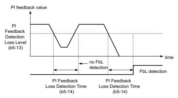
Figure 5.17 PI Feedback Loss Detection
