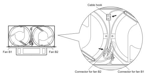
Figure 7.23 Cooling Fan Wiring: 2A0250, 2A0312 and 4A0208
