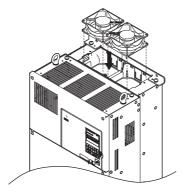
Figure 7.15 Installing the Cooling Fan: 4A0088 and 4A0103
