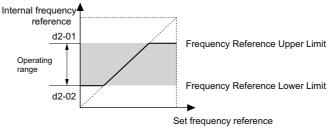
Figure 5.25 Frequency Reference: Upper and Lower Limits
