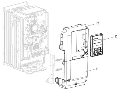
Figure 8.8 Replace the Front Covers and Digital Operator
