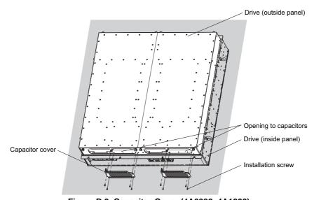
Figure D.9 Capacitor Cover (4A0930, 4A1200)
