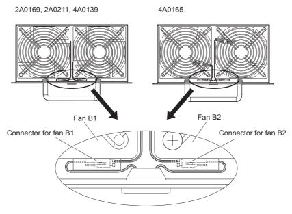
Figure 7.22 Cooling Fan Wiring: 2A0169, 2A0211, 4A0139 and 4A0165
