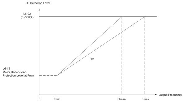
Figure 5.80 Motor Underload Protection
