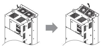
Figure 7.7 Removing the Cooling Fan Cover: 2A0110 and 2A0138, 4A0058 and 4A0072
