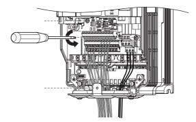
Figure 7.57 Drive Replacement: Removing the Terminal Board
