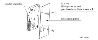
Figure 2.9 External/Face-Mount Installation
