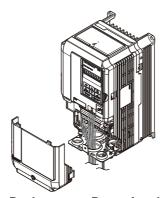
Figure 7.56 Drive Replacement: Removing the Terminal Cover
