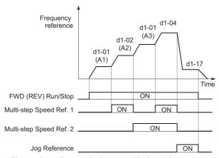
Figure 5.24 Preset Reference Timing Diagram
