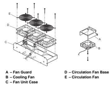
Figure 7.28 Fan Unit Disassembly: 4A0414
