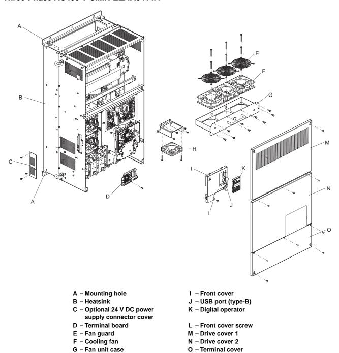
Figure 1.6 Exploded view of IP00 Enclosure Type Components (CIMR-E□4A0414A)
