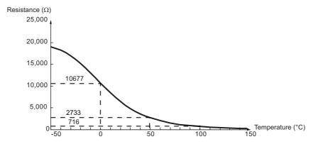
Figure 5.65 Temperature and Resistance of NTC Thermistor
