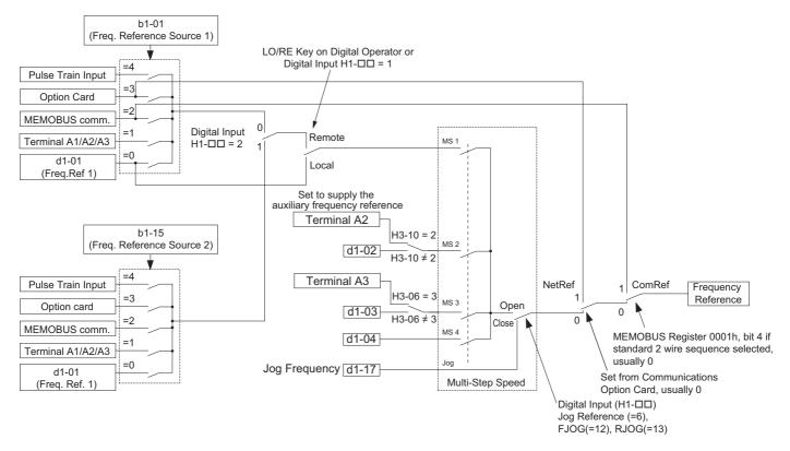
Figure 5.23 Frequency Reference Setting Hierarchy
