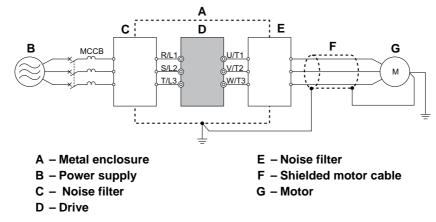
Figure 8.17 Reducing Radio Frequency Noise
