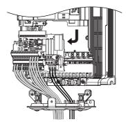
Figure 7.58 Drive Replacement: Remove the Terminal Board
