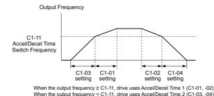
Figure 5.20 Accel/Decel Time Switching Frequency
