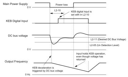
Figure 5.66 KEB Operation Using a KEB Input
