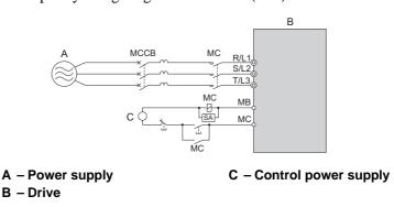
Figure 8.11 Power Supply Interrupt Wiring (Example)
