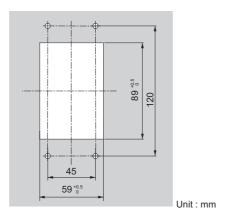
Figure 2.12 Panel Cut-Out Dimensions (Internal/Flush-Mount Installation)
