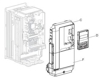
Figure 8.3 Remove the Front Covers and Digital Operator
