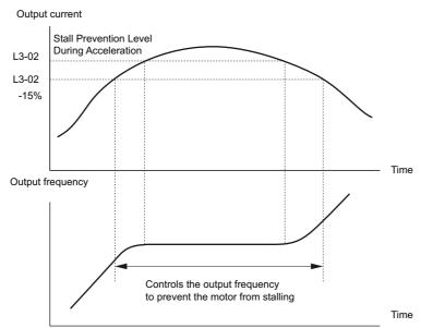
Figure 5.72 Stall Prevention During Acceleration for Induction Motors
