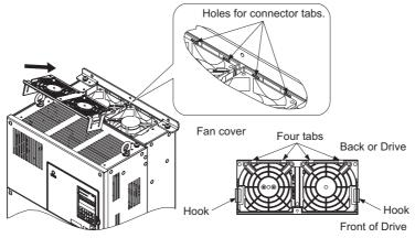
Figure 7.17 Reattach the Fan Cover: 4A0088 and 4A0103
