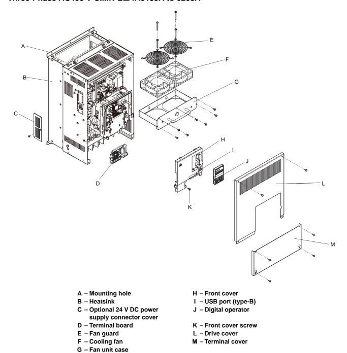
Figure 1.4 Exploded view of IP00 Enclosure Type Components (CIMR-E□4A0165A)
