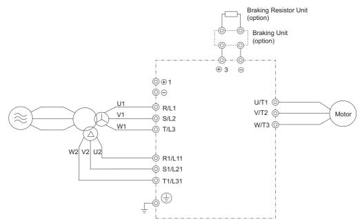
Figure 3.3 Connecting Main Circuit Terminals
