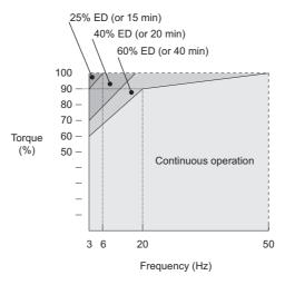
Figure i.2 Allowable Load Characteristics for a Yaskawa Motor
