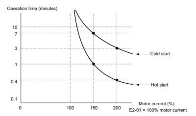
Figure 5.61 Motor Protection Operation Time
