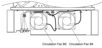
Figure 7.37 Cooling Fan Wiring: 4A0515 and 4A0675
