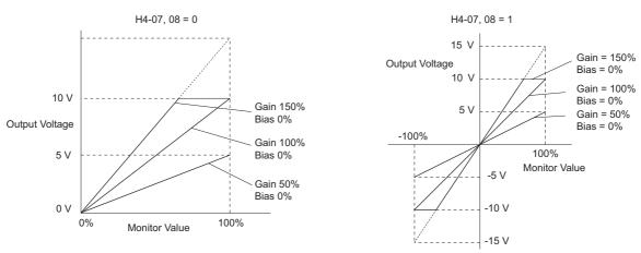
Figure 5.58 Analog Output Gain and Bias Setting Example 1 and 2
