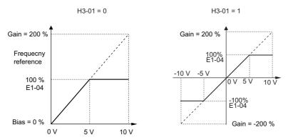
Figure 5.53 Frequency Reference Setting by Analog Input with Increased Gain
