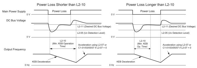
Figure 5.69 KEB Operation Using L2-10, Without KEB Input
