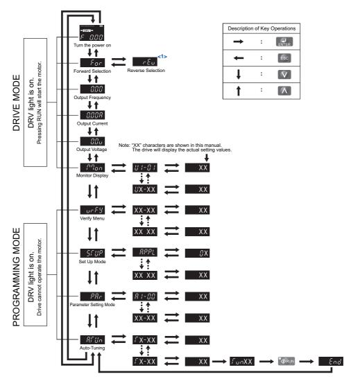
Figure 4.4 Digital Operator Menu and Screen Structure
