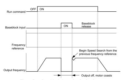
Figure 5.33 Baseblock Operation During Run
