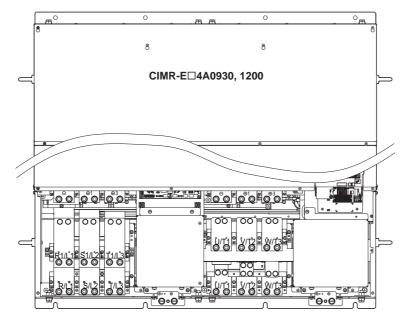
Figure 3.4 Main Circuit Terminal Block Configuration
