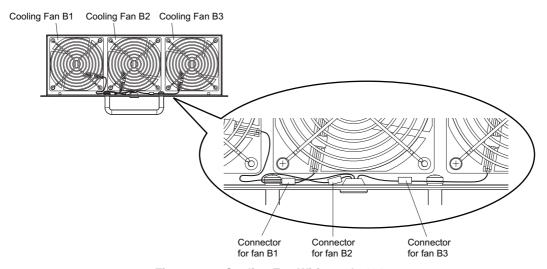
Figure 7.29 Cooling Fan Wiring: 4A0414
