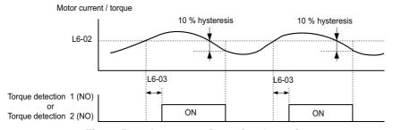
Figure 5.78 Overtorque Detection Operation
