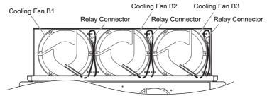
Figure 7.35 Cooling Fan Wiring: 4A0515 and 4A0675
