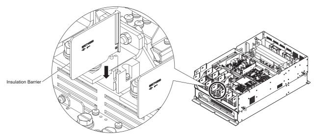
Figure 3.19 Installing insulation barriers
