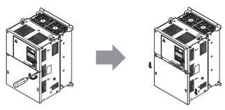
Figure 3.8 Removing the Terminal Cover on an IP00 Enclosure Drive
