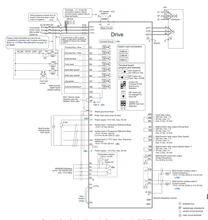
Figure 3.1 Drive Standard Connection Diagram (example: CIMR-E□2A0040)
