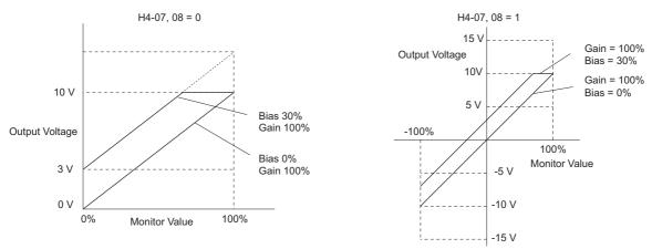
Figure 5.59 Analog Output Gain and Bias Setting Example 3
