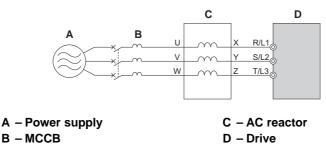
Figure 8.12 Connecting an AC Reactor
