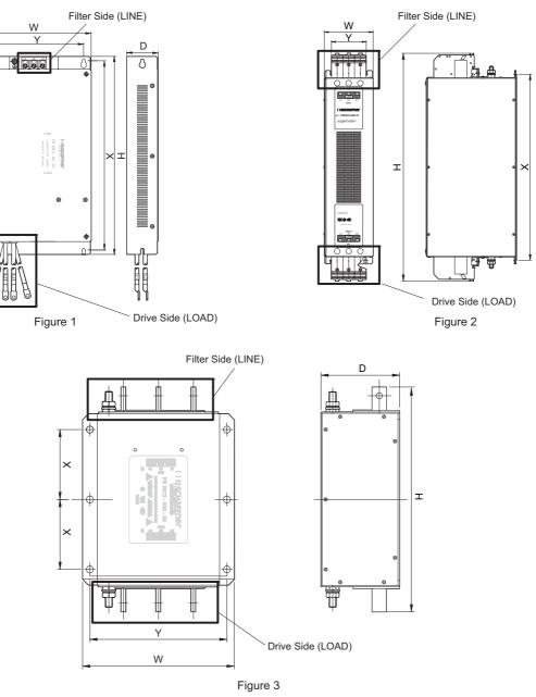
Figure D.5 EMC Filter Dimensions
