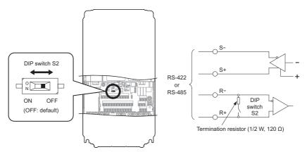
Figure C.5 Serial Communications Terminal and DIP Switch S2
