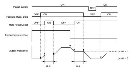
Figure 5.27 Frequency Reference Hold with Accel/Decel Hold Function
