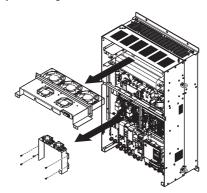
Figure 7.33 Removing the Fan Units: 4A0515 and 4A0675
