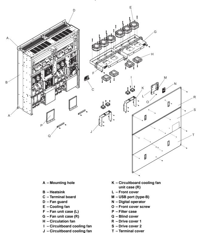
Figure 1.8 Exploded view of IP00 Enclosure Type Components (CIMR-E□4A0930A)
