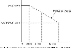
Figure A.4 Carrier Frequency Derating (CIMR-E□4A0139 to 4A0362)
