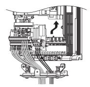
Figure 7.60 Drive Replacement: Installing the Terminal Board
